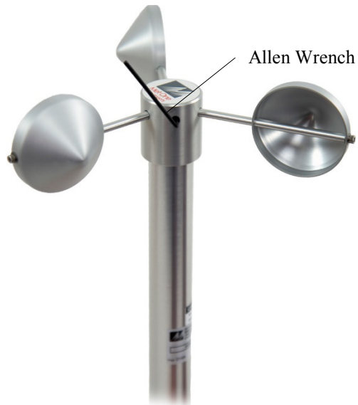
FIGURE 7-2. Allen wrench tightening bolt
